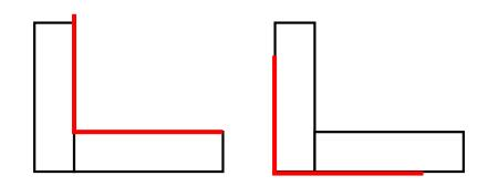
Internal and external waterproofing/tanking waterproofing film, or paintng rubber/tar...
