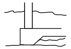
Rafts are slabs that cover a wide area, often where gorund conditions are poor. runs whole length of building, pockets of sand and gravel on the interior, has reinforcing rebar/wire mesh.
