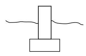
pad foundations: rect or circ to support localized loads, like columns
